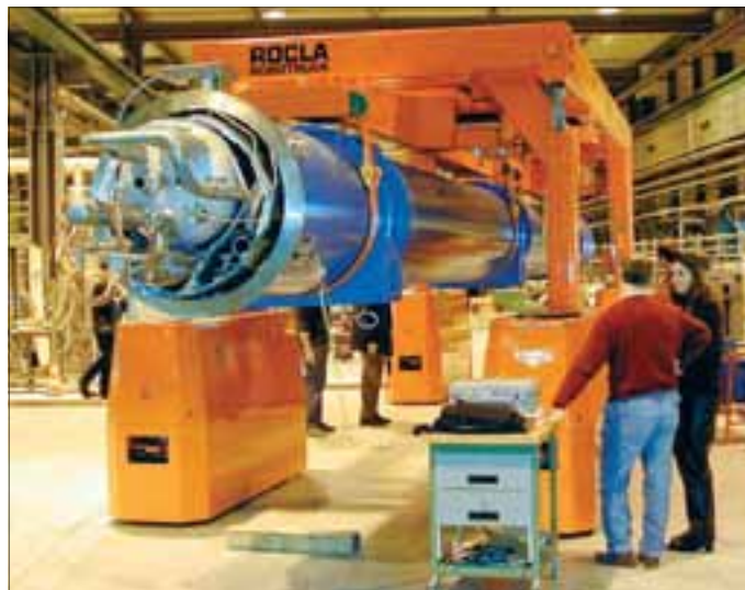
The LHC uses more than 1200 dipole magnets to bend protons around its 27 km circumference.
