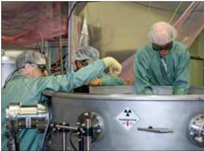
Researchers inserting a target assembly into the PHELIX laser beamline at the GSI lab in Darmstadt. Earlier this year, the LIGHT team connected the laser-ion-acceleration target chamber to an existing ion-accelerator beamline at the lab.
