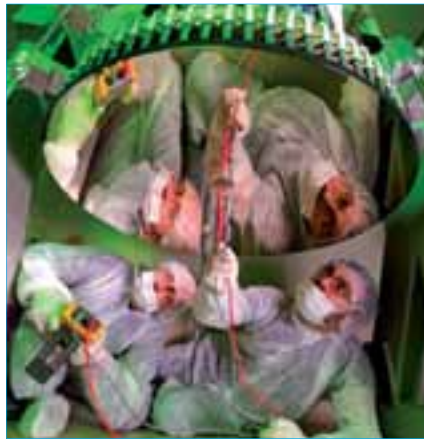
Researchers test the adaptive-optics mirror for the Large Binocular Telescope based in Arizona.
