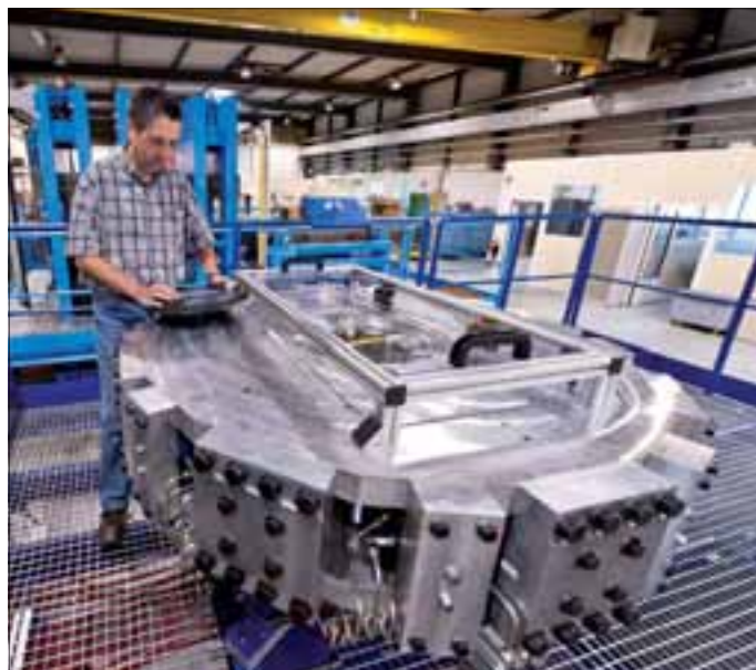
Testing a new type of quadrupole magnet that will be used in a future upgrade of the Large Hadron Collider at CERN.
