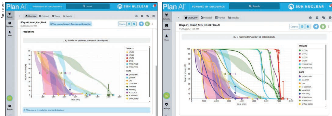
Left: Plan AI software Comparing dose–volume histogram prediction bands with clinical goals (arrows) provides users with valuable feedback on what can be achieved. Right: Clinical plan The screen shows a review of the results that the treatment planning system achieved, with dose–volume histograms shown by the solid lines.
