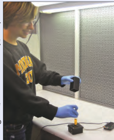
Printable lab equipment A student tests the 3D-printed analyser.
