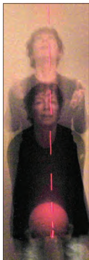
Of! A person catches a 5 kg medicine ball dropped from about 1 m. A blinking LED shows the time interval of the catch.
