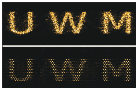
Localization in action Simulation of image carried by the new fibre (top) and a conventional fibre.
