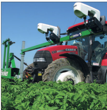
Physics in the field Tractors fitted with commercial optical sensors can reduce the use of pesticides.
