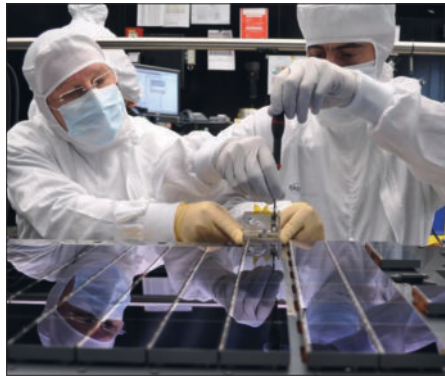
Billion-pixel camera Gaia's optical plane uses 106 high-performance CCDs to convert faint starlight into electrical signals, which will be processed and beamed back to Earth at a rate of about 10 Mbits/s.
