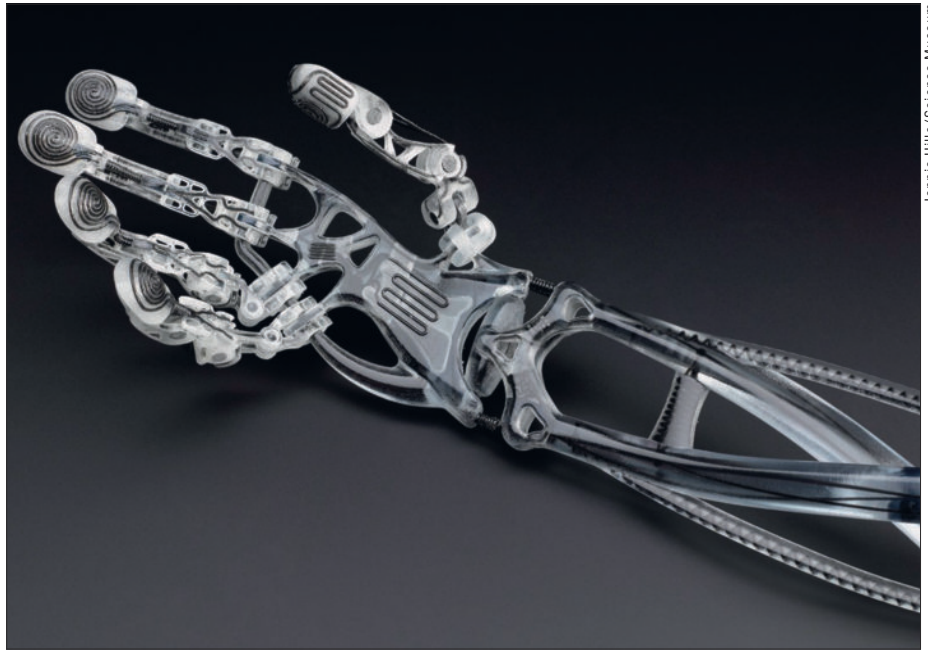
Handy tool A 3D-printed functionalized prosthetic arm with electronic parts and nerve endings fabricated at the University of Nottingham.
