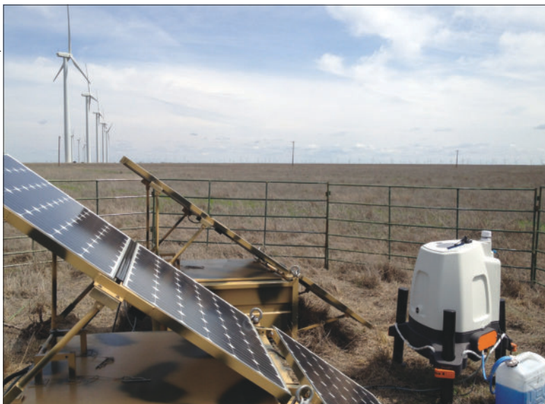
There she blows A portable lidar unit can be moved across a wind farm to analyse wind patterns and improve turbine alignment.
