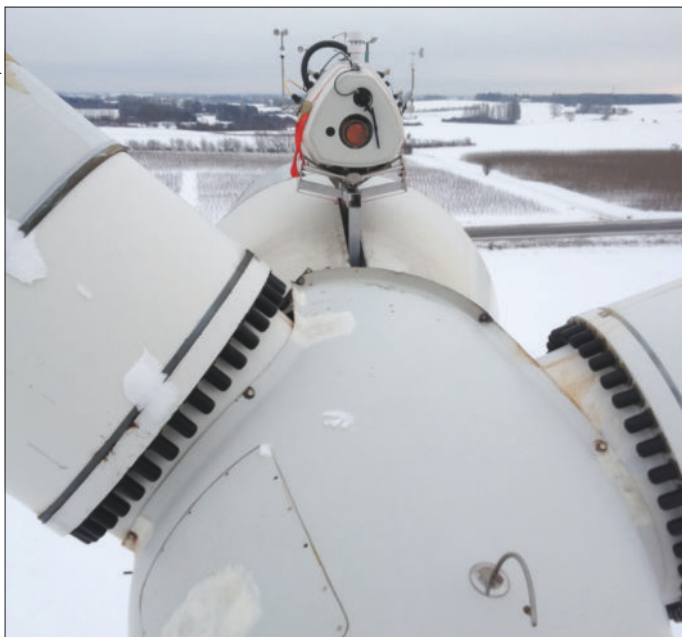
Planning ahead Mounting a lidar unit on the turbine itself allows it to detect turbulence up-wind and prepare the blades in a less-resistant pitch.
