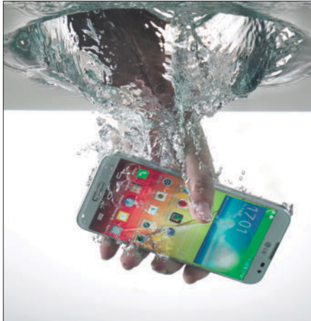
Off you go A nanoscale polymer film deposited on mobile devices makes water bead and roll off.
