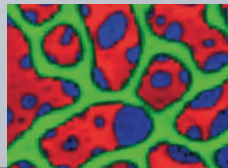
Confocal Raman and AFM topography image of a polymer blend on glass
