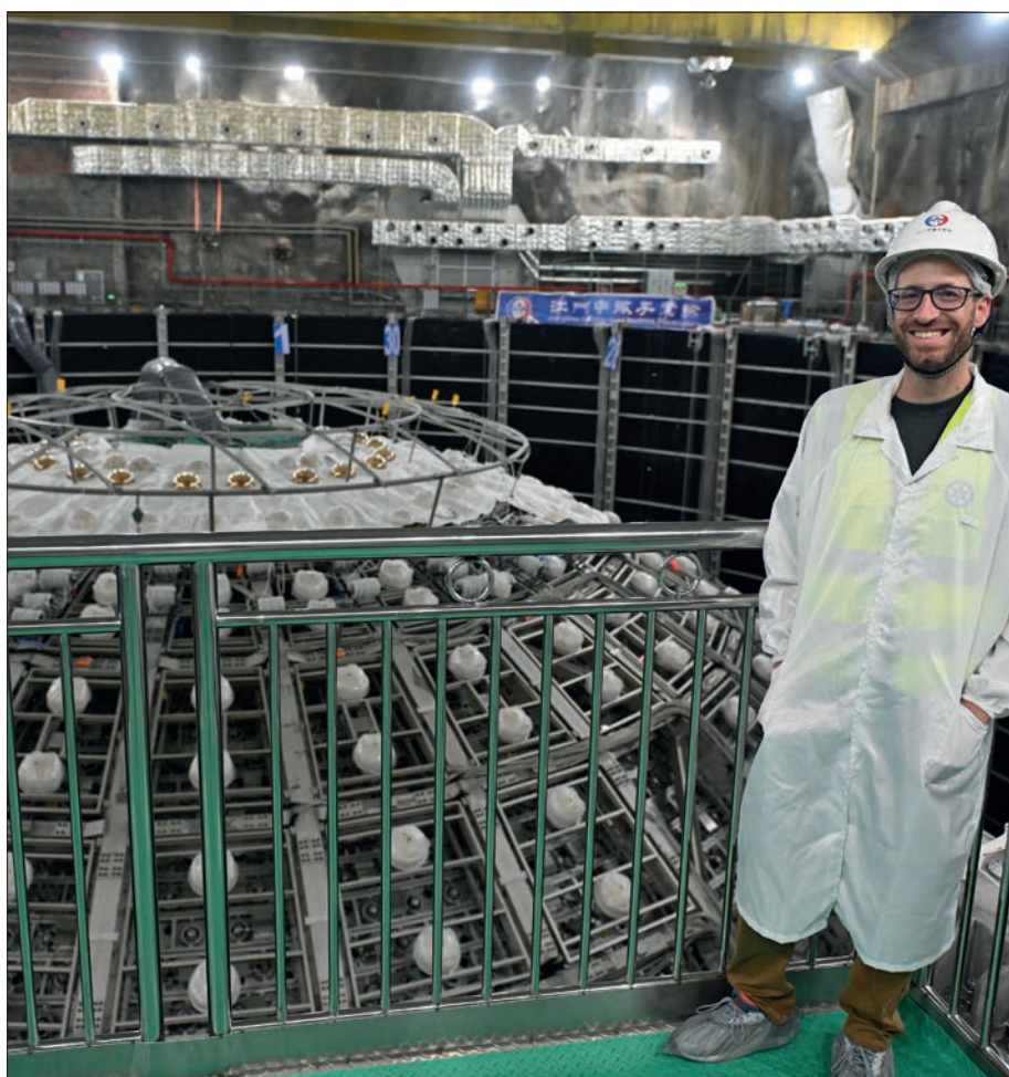
Science at work Juan Pedro Ochoa-Ricoux at the Jiangmen Underground Neutrino Observatory (JUNO) during its construction. Ochoa-Ricoux stands in front of the detector, a 35.4 m diameter sphere filled with 20 kilotons of liquid scintillator that will study neutrinos from nuclear reactors.
