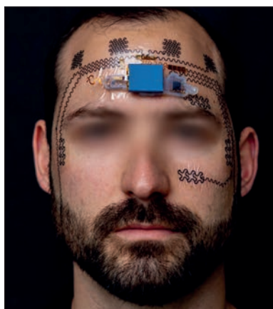
Skin deep The e-tattoo can carry out electroencephalography and electro-oculography via adhesive electrodes with a flexible printed circuit module.
