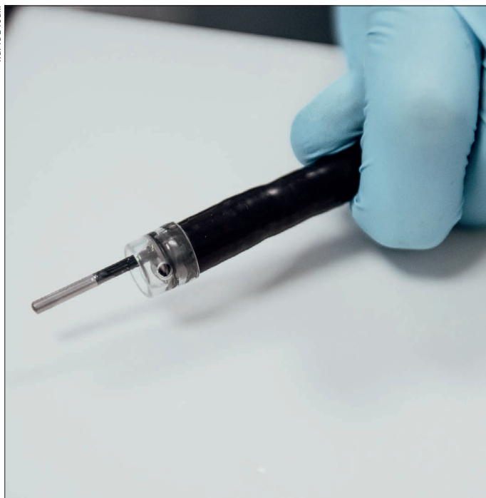
Tiny but mighty (above) A Raman probe protruding from the instrument channel of an endoscope. (right) Oliver Old, consultant surgeon, passing the probe down an endoscope for a study led by the University of Exeter, with the University of Bristol and Gloucestershire Hospitals NHS Foundation Trust as partners.
