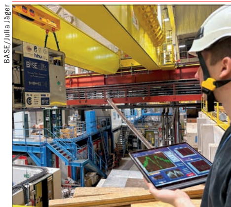
The BASE-STEP autonomous Penning-trap system is moved to a lorry at CERN. The system could soon be used to move antimatter p27
