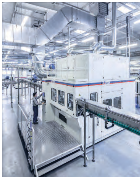
Bottling benefits The Van Pur brewery in Poland uses plasma impulse chemical vapour deposition under vacuum (in a facility supplied by KHS Plasmax) to coat the insides of bottles with an ultrathin layer of glass.
