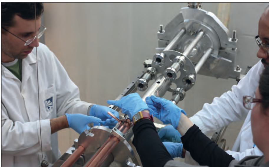
High production Intertwisted titanium, zirconium and vanadium wires being assembled into Sirius vacuum chambers in the NEG-coating rig at the Brazilian Light Source Laboratory. These are then inserted into a solenoid where a DC magnetron sputtering process completes the coating process. When fully loaded, the rig can simultaneously coat six 3.2 m-long vacuum chambers.
