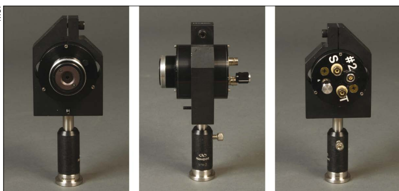
Candela In the 1990s NIST used this silicon diode photodetector, which included a filter that spectrally matched the accepted human visual response, to realize the candela. This was the first use of a detector device to realize the candela for the US.
